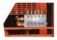
8. Hydraulic Transmission Hydraulic transmission for vibration bar, stepless frequency conversion to supply optimum frequency for all types of concrete.
