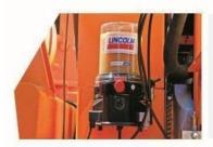
6. Centralized lubrication Automatic centralized lubrication system – effectively improve the reliability of the Tamper and feeding
