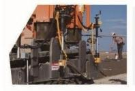
3. Auto Levelling System Auto levelling and tracing system to ensure paving surface flatness and road straightness
