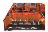
4. Scraping "Plate Controlled by two hydraulic cylinders to control the incoming concrete quantity to the shaping template. The level of the scraping plate is automatically adjusted on both LH and RH independently.
